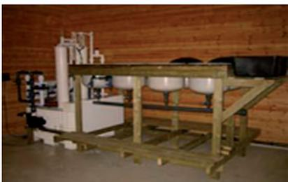
Larvae hatch in specially designed and fully scalable recirculating hatcheries that allow improved control of water parameters and biosecurity.
